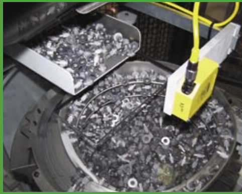
Feeder Bowl with Level Sensing
